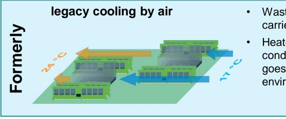
• Waste heat of processors and memory carried off by cool air
