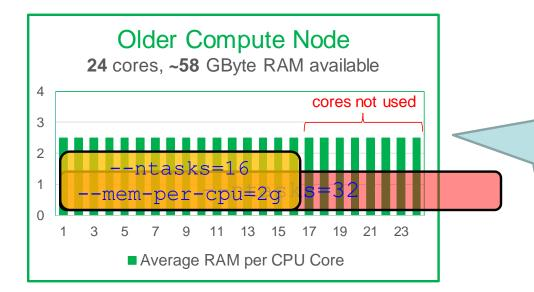
Older node with 24 cores taken *just as an example* – 96 cores would "detonate" this figure to be unreadable. Transform the principle to 96 cores and ~4096 MByte/core
