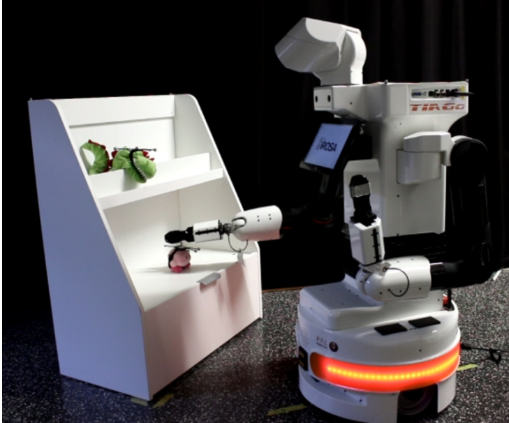
Figure 1: Real Tiago robot safely interacts in a real-world environment, while avoiding collision with complex geometries
